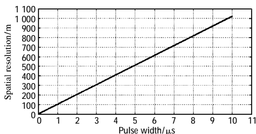
Fig. 3 Relationship of the spatial resolution with pulse width
