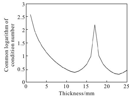
图 4 Savart 单板厚度  $t$  与条件数  $\kappa$  之间的关系Fig.4 Dependence between the thickness  $t$  of the Savart plate and the condition number  $\kappa$
