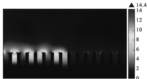
Fig.6 Corresponding electric field distribution of spoof SPPs for h_1=100\ \mu\text{m} , based on the Fig.5 model
