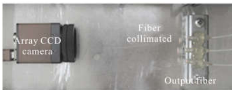
Fig.5 Stability testing of the system based on the collimated beam
