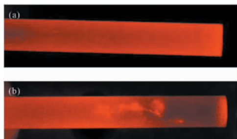
Fig.8 Comparison between damage and no damage in Nd:YAG rod
