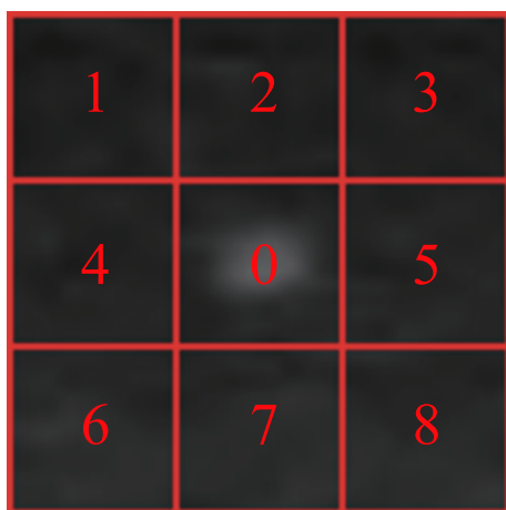
Fig.2 A local small image patch used for MRDLCM calculation. It is divided into 9 cells, and the cell size N should be close to or slightly larger than real target
