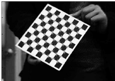
图 10 畸变补偿后的第 7 幅图角点提取效果 Fig.10 Corner extraction result with distortion compensation
