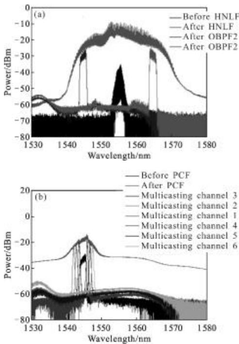
Fig.5 (a) Optical spectrum measured at the input, the output of 700-m HNLF and the output of OBPF2, (b) Optical spectrum measured at the input, the output of DF-HNL-PCF, and the output of OBPF3 for  $\lambda_{\text{signal}}=1545\text{ nm}$
