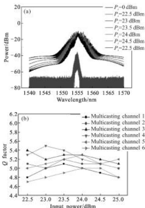
Fig.6 (a) SPM broadened spectrum of RZ signal for different input signal power, (b) Q factor versus input signal power for 6 multicasting channels
