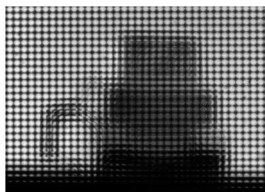
Fig.7 Raw image of a toy car when the applied voltage signal is ~5.0 Vrms
