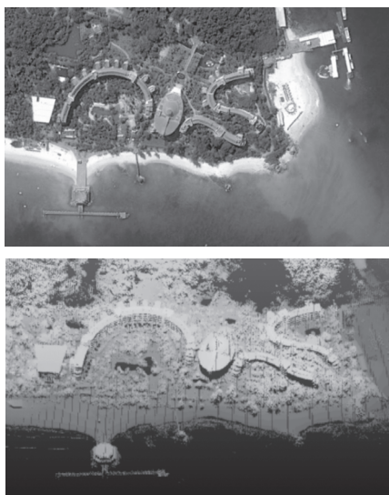
图 7 蜈支洲岛卫星图片和双频激光雷达三维点云图对比 Fig.7 Satellite image of Wuzhizhou Island versus point cloud image of Wuzhizhou Island produced by dual-frequency lidar
