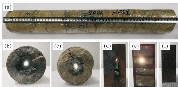
图 10 砂岩激光射孔的侧面(a)、入射面(b)及出射面(c)照片，钢板激光射孔的入射面(d)、出射面(e)及侧面(f)照片 Fig.10 Photographs of the side (a), incident surface (b) and exit surface (c) of the sandstone after laser perforation, photographs of the incident surface (d), exit surface (e) and side (f) of the steel sheet after laser perforation
