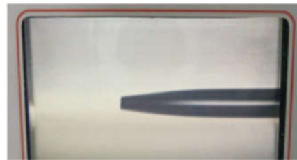
Fig.13 Effect diagram after HCPCF taper cutting
