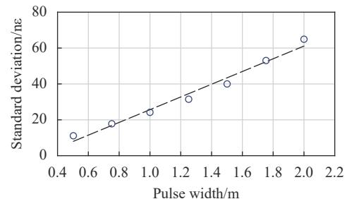
图 4 应变水平标准差和脉冲宽度数值模拟<sup>[11]</sup>Fig.4 Numerical simulation of standard deviation of the strain level and pulse width<sup>[11]</sup>
