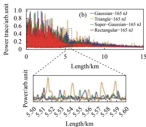
图 6 不同脉冲形状下散射曲线能量曲线及局部放大图<sup>[14]</sup>Fig.6 Backscattering power traces from different pulse shapes with magnification of traces<sup>[14]</sup>
