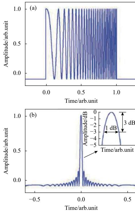
图 12 线性频率调制光脉冲。(a) 时域波形;(b) 压缩后波形<sup>[29]</sup>Fig.12 Linear frequency modulates light pulses. (a) Time-domain profile; (b) Compressed profile<sup>[29]</sup>
