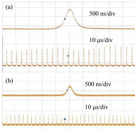
图6 饱和吸收体为(a)MoS<sub>2</sub>和(b)GNCs时获得的单脉冲波形和脉冲序列Fig.6 Single pulse profiles and pulse trains of (a) MoS<sub>2</sub>-SA and (b) GNCs-SA Q-switched Nd:YAG lasers
