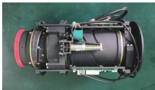
(a) 装配完成的水下变焦镜头 (a) The assembled underwater zoom lens
