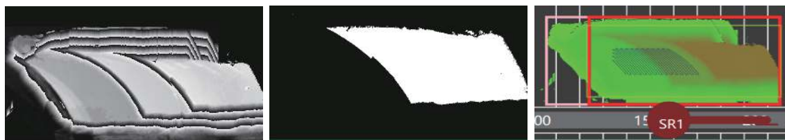
(a) 料堆灰度图 (a) A grayscale image of the stock pile (b) 补堆边界识别 (b) Boundary identification of the patch heap (c) 补堆路径规划 (c) Path planning for making up the heap
